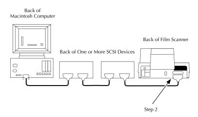
3. Attach the SCSI terminator (supplied with the Scanner) to the empty SCSI port on the Scanner, seat the terminator firmly, and pinch the wire clamps shut.
